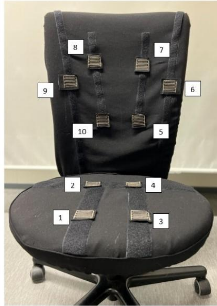
Figure 11 Examples of textile-based pressure arrays and posture-mapping systems for seating [23].
