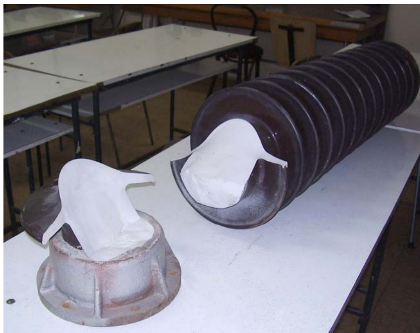
Fig. 3.1. – Ceramic Insulator braked from the metalic bottom support
