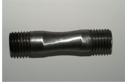
Fig.1. Test specimen from 16Mo5.3b, pending testing
