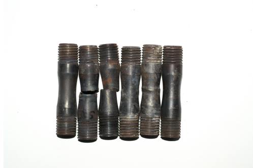
Fig. 2. Test specimens tested to thermomechanical fatigue
