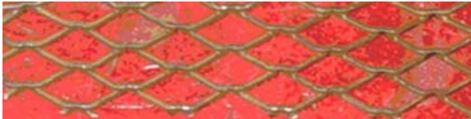
Fig. 2. Plane structure of expanded metal made out of five threads
